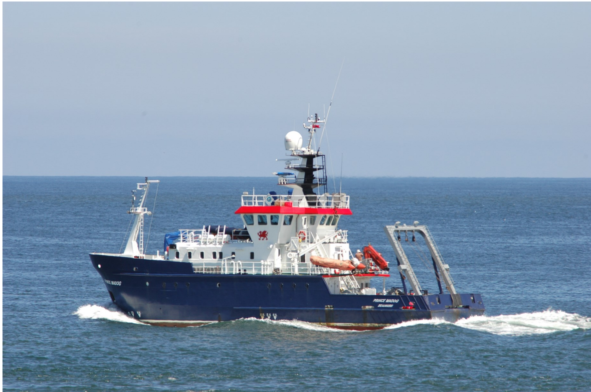
Bangor University's Research Vessel "R.V. Prince Madog" is a state-of-the-art purpose built 35 m research vessel. The vessel travels to the Isle of Man for 2 weeks each year to undertake an annual scallop survey. The vessel is fully equipped for surveying and holds 8 vessel crew and 10 scientists.
