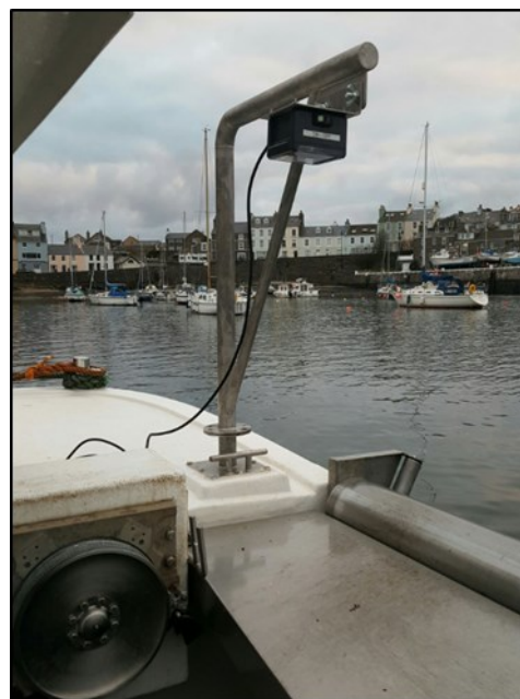
Figure 18: A parallel paired laser onboard FV Shelgeyr, Port St Mary.
