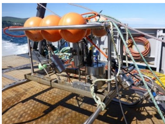
Figure 25: Towed video sledge comprising a stills camera and flash, a live video feed with lights and a mounted GoPro and maps indicating the location of video transects within both Laxey Bay (A) and Niarbyl Bay (B).
