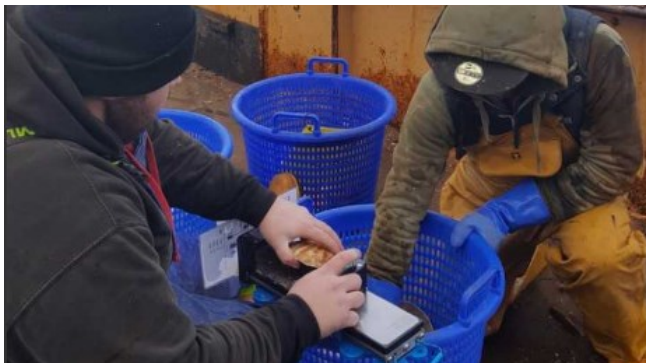
Figure 29: Above: The purchased decklogger being used in trials to record catch and effort data onboard a Manx whelk boat. Left: MFPO scallops survey using the electronic measuring board.
