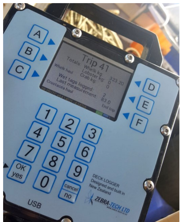
Figure 29: Above: The purchased decklogger being used in trials to record catch and effort data onboard a Manx whelk boat. Left: MFPO scallops survey using the electronic measuring board.
