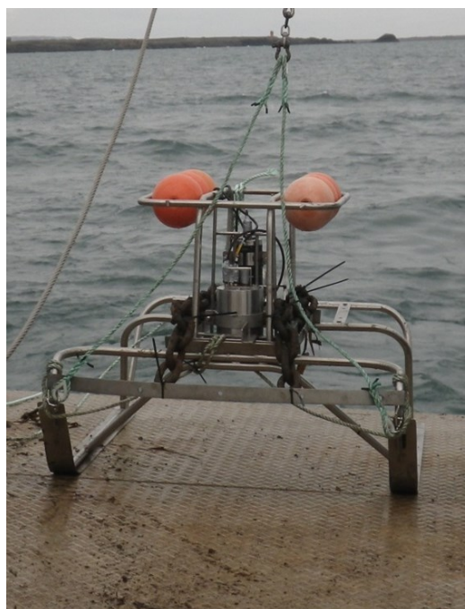
Figure 30. Survey equipment: metal sledge with cameras and underwater lights attached.
