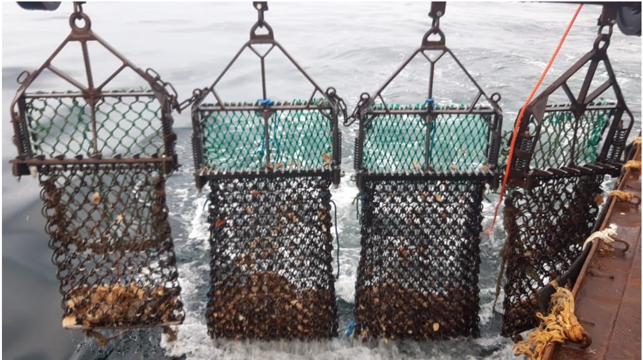
Figure 1: 'Juvenile' survey bar showing the two modified queen scallop dredges in the centre of the bar (17 teeth and smaller mesh) and two standard king scallop dredges on the outside of the survey bar.
