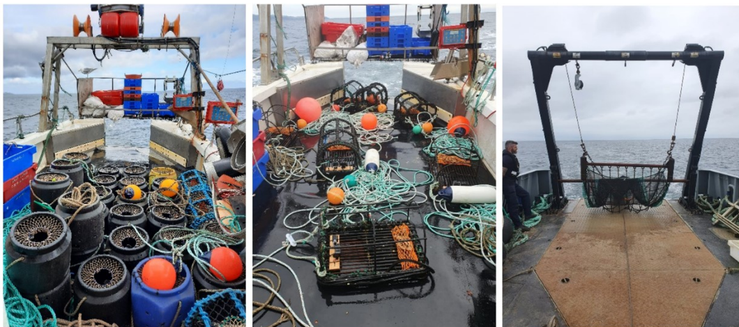
Figure 27. Sampling gears trialled for whelk stock surveys: commercial whelk pots (left); BRUVs (middle); beam trawl (right).
