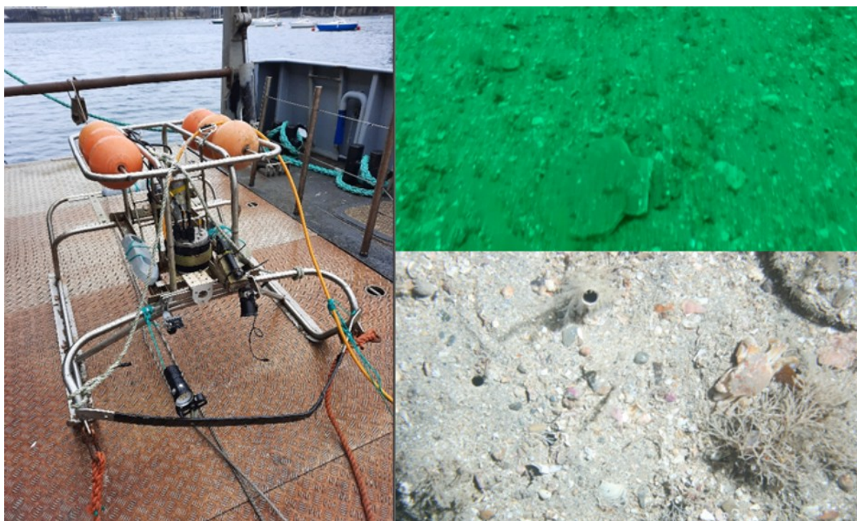
Figure 21: Towed video sled system, a screen shot from the GoPro video used to determine scallop seabed density and still image used to determine habitat type.
