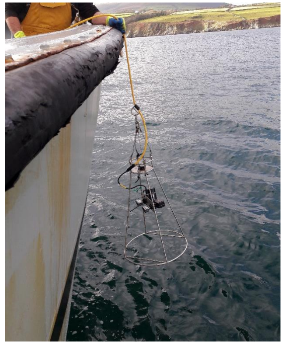
Figure 1: Photograph demonstrating the drop-down camera setup used to collect benthic video footage in Baie ny Carrickey MNR.
