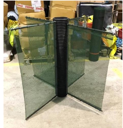
Figure 3. “X-shaped” spat receptor model tested in EDG ERA, inspired by the design of Fegley et al. (2009).
