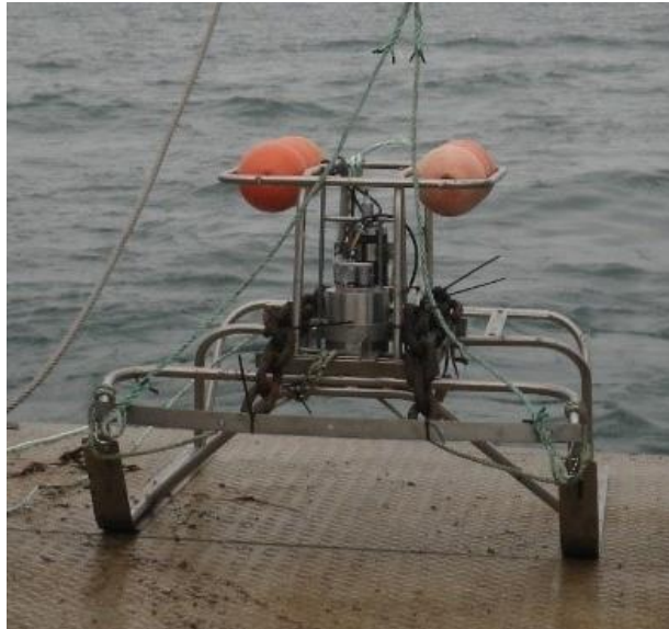
Figure 2: Photograph of the equipment used to collect benthic image data, designed to “ski” along the seabed with minimal damage. Cameras and lights were attached to the central raised unit.
