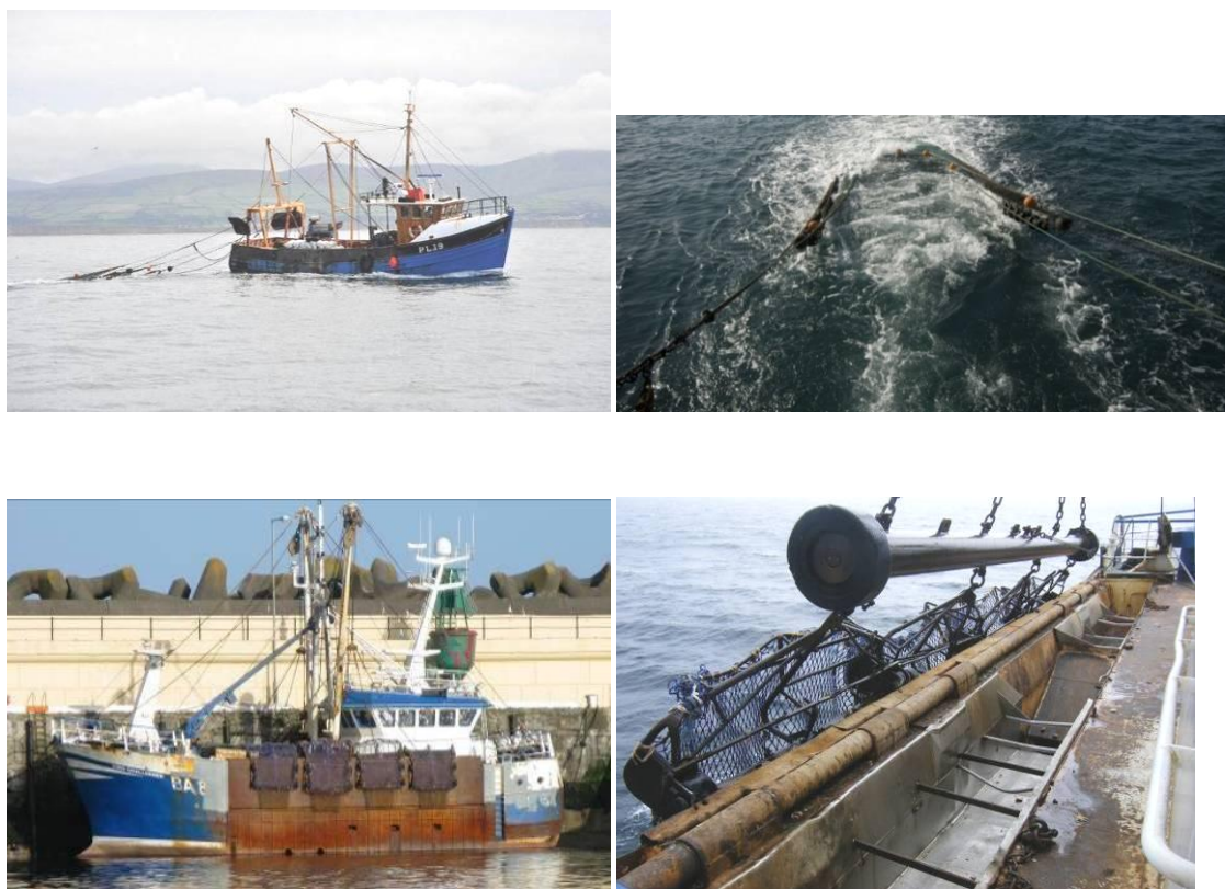
Figure 1. Typical trawling vessel and otter trawl (top) and one of three dredging vessels and toothless dredges (bottom) used to fish for Aequipecten opercularis around the Isle of Man.
