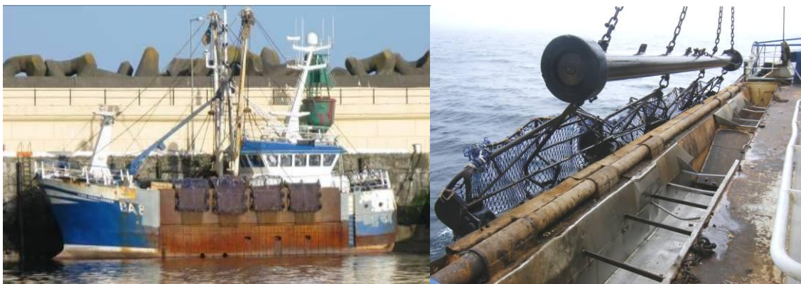
Fig 6. King Challenger in Douglas Harbour after the gear trial with New dredges hanging over the side and during fishing operations at sea.
