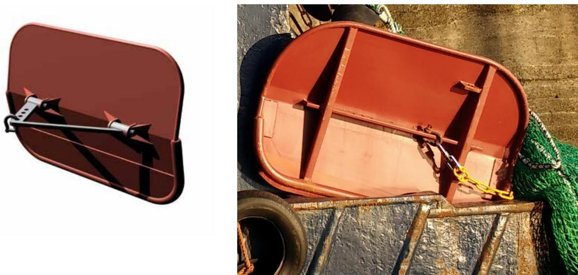
**Appendix 3.** Otter board doors. Left – illustration of a typical Steel V door (Seafish, 2015); Right – a photograph of one of the Dunbar V doors used on the vessels *Two Girls* and *Our Sarah Jane* in the commercial gear trials.
