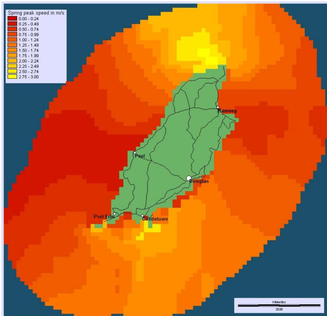
*Appendix 1. The spring peak tidal stream speeds (m/s) in Manx waters, with areas of slowest flow rate indicated in red and fastest in yellow (Aguatera 2006).*
