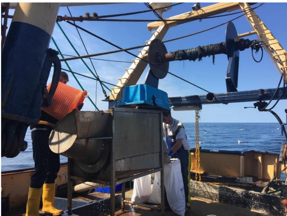
*Appendix 7 Queen scallop catch being poured into the mechanical riddle, to mechanically sort the undersized (<55mm) individuals from the oversized marketable catch which is subsequently retained in commercial sacks ready to be landed (photograph taken on board Two girls during the bycatch trials 2017).*
