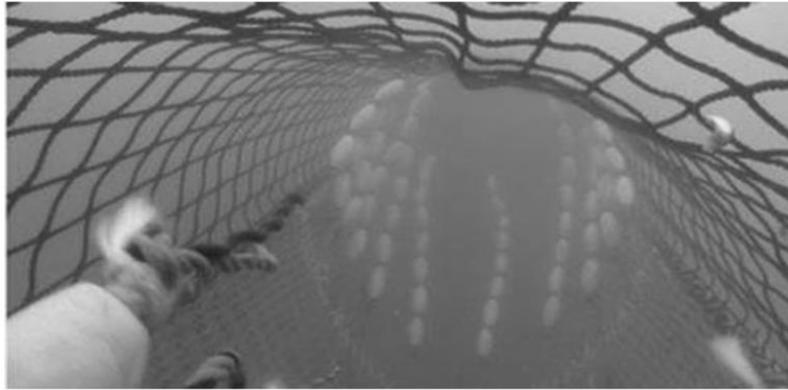
**Figure 26** Image of the float ropes used to guide fish, such as cod to swim up towards the SMP rather than remaining low in the net. This photo is taken during towing at a speed of three knots. The image is taken at the front part of the codend looking towards the aft end. (Herrmann *et al.* 2015)
