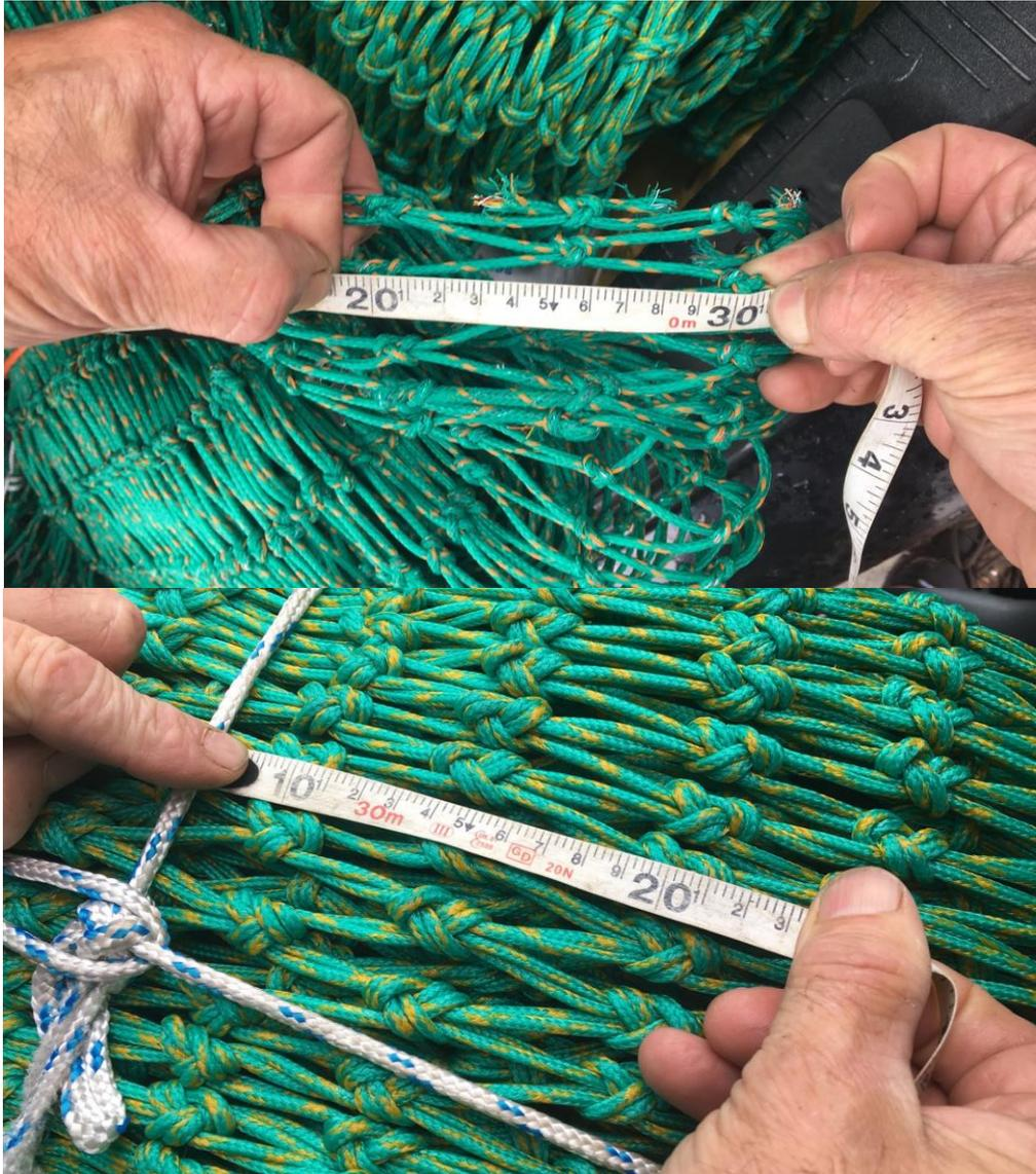
**Appendix 2.** Photograph of the diamond mesh measured from knot to knot: top photo – single twine meshes used in the top section of the net; bottom photo – double twine used in the bottom section of the net.
