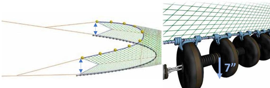
**Figure 5** Illustration of a 'square set' fish tail, with the headrope and footrope set directly above one another (Left) and; the rock hopper footrope, illustrating the height in which the footrope gear is towed above the seabed (Right) (Adapted from, Seafish 2015).
