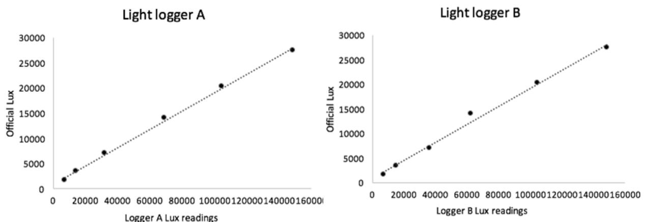
**Figure 6** Calibration coefficient for both HOBO loggers used in the survey (logger A and B), with the official lux readings recorded using a calibration light meter, correlated against the readings recorded by the loggers.
