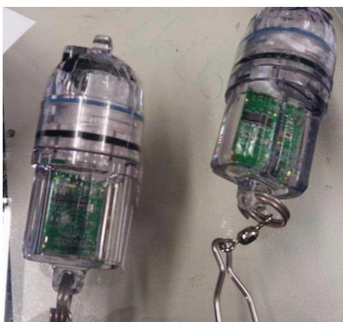
*Appendix 8 HOBO UA-002-64 64K Pendant Temp/Light Loggers (Tempcon Ltd) (left) and the HOBO loggers inserted into the SafetyNet Technologies Ltd. housings made originally for LED lights, as they can withstand higher pressure in comparison to the original HOBO casings (Right).*
