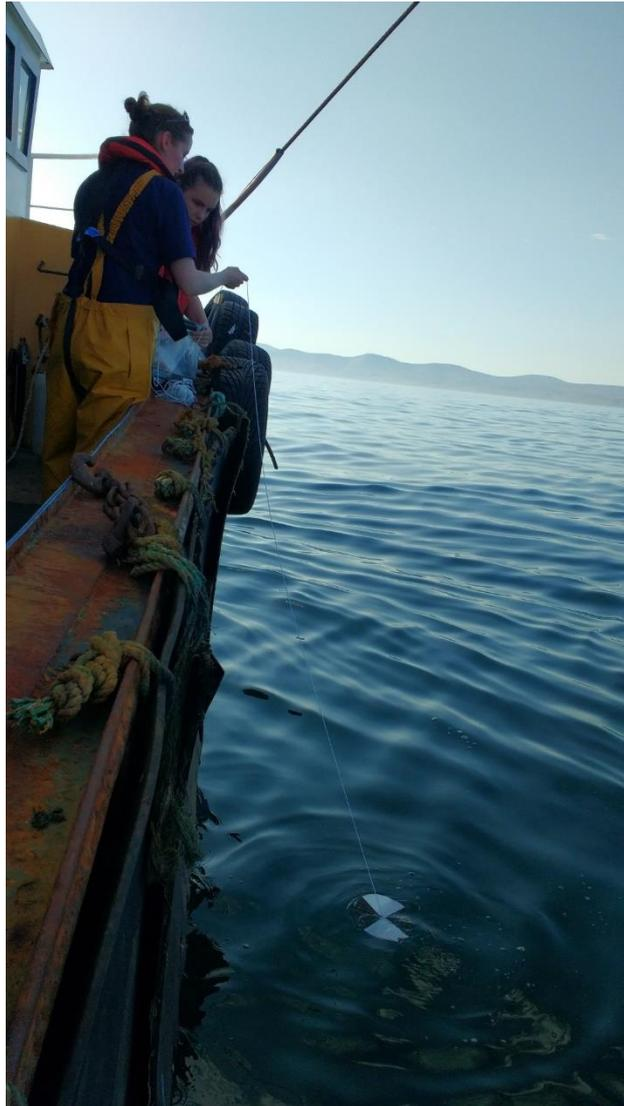
*Appendix 9* A photograph demonstrating the procedure used to measure water turbidity, using a Secchi disk which was lowered into the water column until it was no longer visible and then the number of notches (1 every metre) were counted as it was hoisted back on board the vessel, during the bycatch trials in IoM waters.
