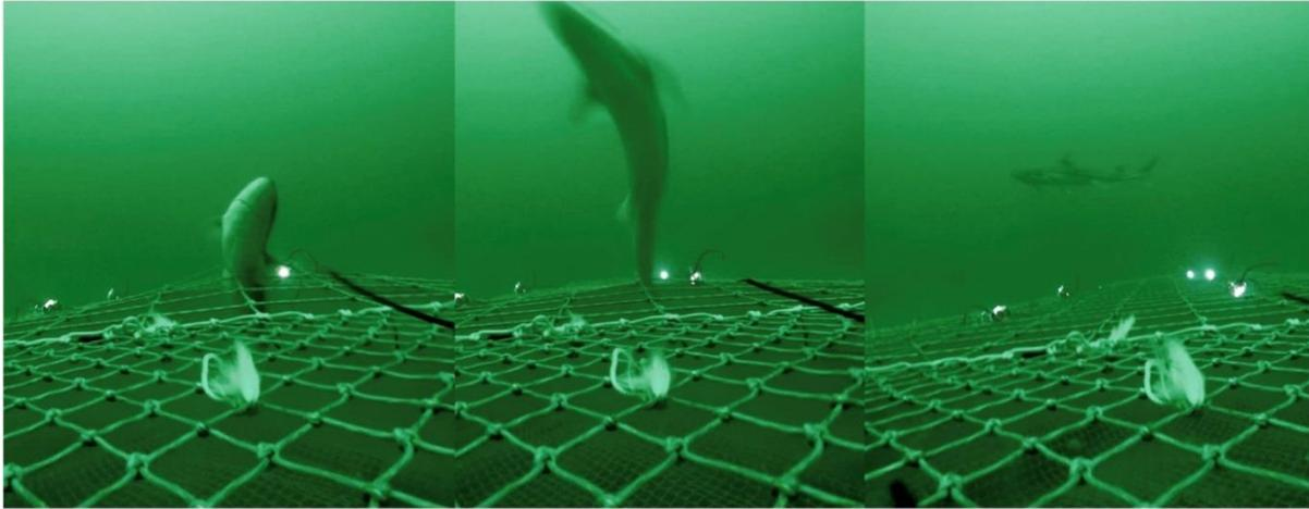
**Figure 25** Stills from the GoPro video footage of a shark species escaping through the large meshes in the square mesh panel implemented into the queen scallop otter trawl, in the IoM. The image is taken from the top of the net anterior to the square mesh panel on the outside of the net looking towards the aft end of the net.
