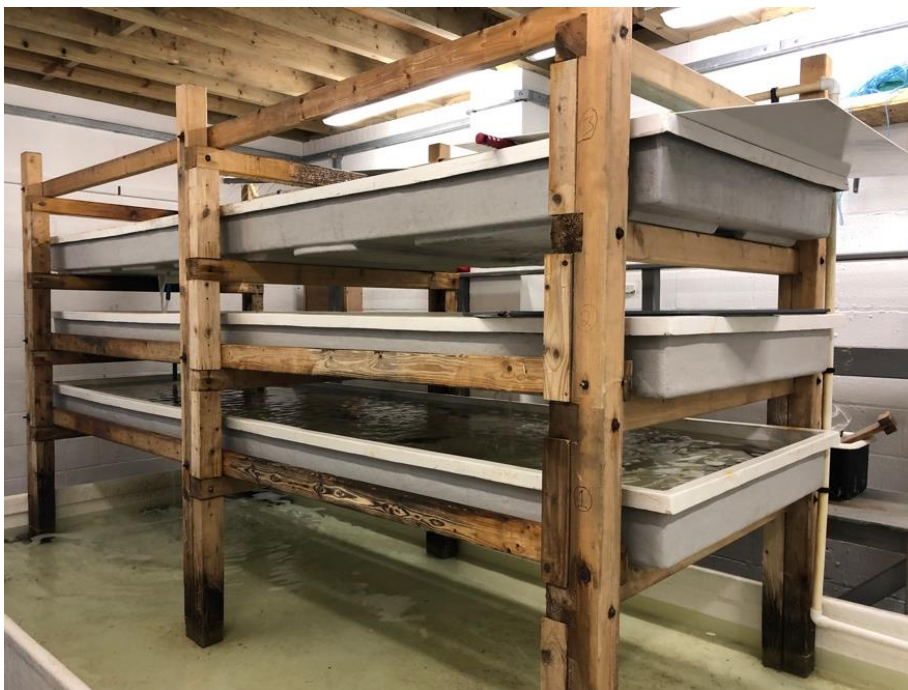
Figure 9 Holding tank setup at Lewis Seafood in Peel. The top three layers of the tanks will be used for plaice survival observations. Each tank layer measures 418 x 114 x 16 L x W x D (cm). The tank uses a recirculating sea water system with cascade flow, a protein skimmer and bio filter.
