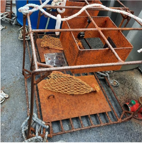
Fig. 4. Photograph of the BRUVS, equipment used for collecting mobile species data. Three GoPro cameras at different viewing angles were fixed on top of the rectangular metal frame.
