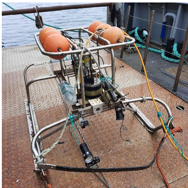
119 120 Fig. 3. Photograph of the equipment, the sledge, used for collection of the benthic imagery data. Both the cameras and 121 light were fixed on the raised unit at the centre.
